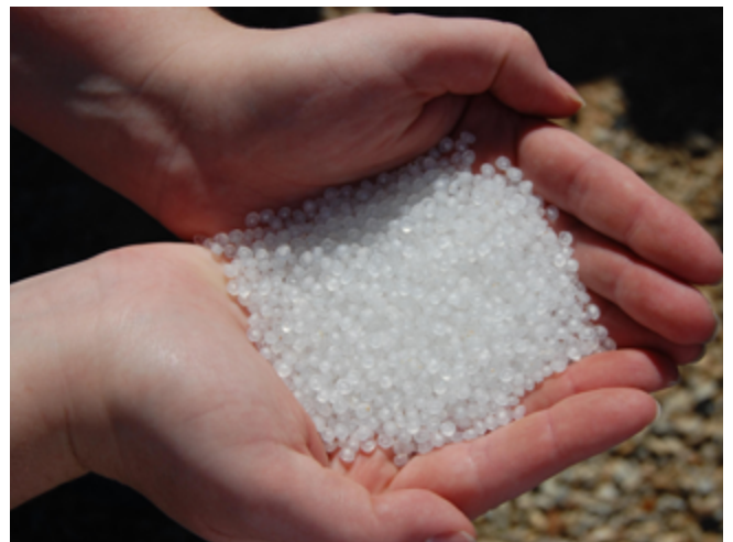
Nurdles that spilled from a train in the USA Image credit: gentlemanrook via Wikipedia
